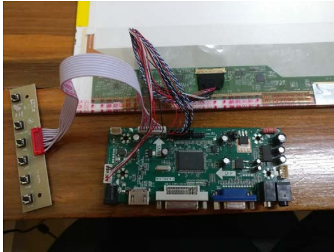
Figure 3: LCD Control board and LVDS cable.
