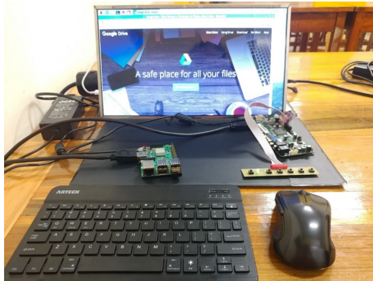
Figure 2: Fully assembled Raspberry Pi workstation with wireless mouse and Bluetooth keyboard.
