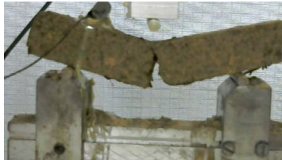
Figure 4: A sample of Piarco soil at failure. Sample number S4 with 4% peat, 24% moisture content at 10 Hz
