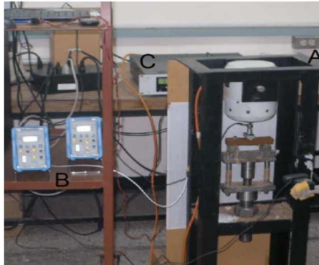
Figure 1: Physical arrangement of Dynamic Tester (A), Signal processors (B) and Amplifier (C)
